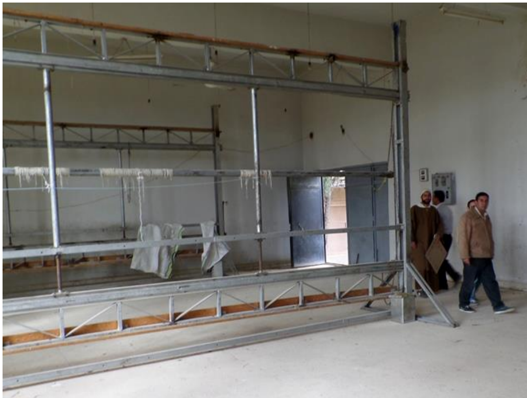
This is their biggest machine: here they can make carpets of with width of seven meters. For the presidential palace this factory boasts to have made a carpet on this machine of 25m long.
